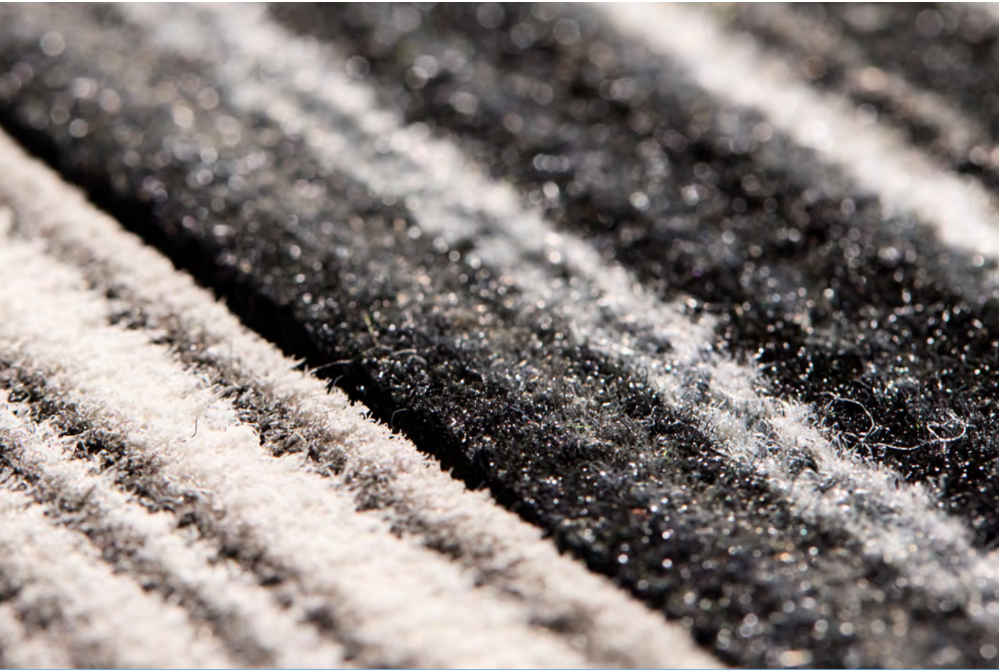
Fiber glass is added to ensure excellent dimensional stability and durability
